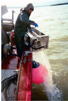
Figure 9 Live box, or recovery box <sup>49</sup>
